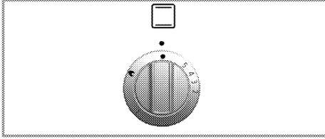
Grill is operated with Grill control knob. In turned off position (top), gas is not supplied. Oven door must remain open while grilling.
